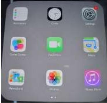
**GUI, graphical user interface:** A type of user interface that allows users to interact with electronic devices with images rather than text commands. A GUI represents the information and actions available to a user through icons. Pronounced *Goey*.
