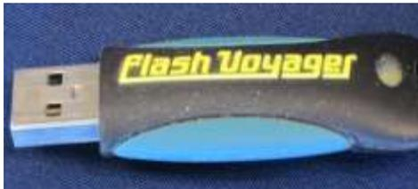
**Flash/thumb drive:** A portable storage device that connects to a computer with a USB connection.
