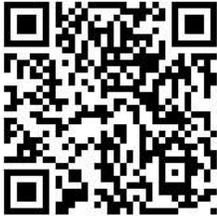
**QR, quick response codes:** A type of barcode that consists of a printed square pattern of small black and white squares that represent numbers and letters. The codes are read with laser scanners, cameras, or smart phones. They are most often used in advertising to encode an Internet address.
