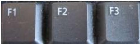
**Function keys:** Normally, at the top of the keyboard are 12 keys that are numbered with an F in front of them. These keys can be set up to carry out a function within a module or computer program. For example, in Workflows, F5 is checkout.
