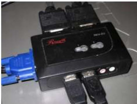
**KVM switch:** A device that allows a single keyboard, video monitor and mouse to control more than one computer at a time.
