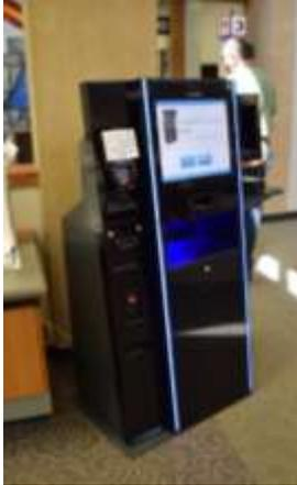
**Selfcheck:** Library users can check out items for themselves without staff assistance using the software and supporting hardware. Generally there is an infrared scanner to read the user barcode, bring up the record, and scan the item's barcode or RFID code
